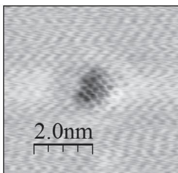
Figure 2: Atomically resolved STM image of suspended graphene.
