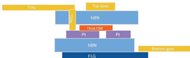
Figure 3: Transverse view of the device "stack", with colors corresponding to Figure 2.
