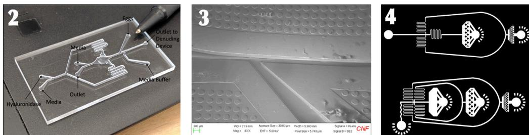
Figure 2, left: Acrylic microfluidic device aimed at exposing and separating the COCs. Figure 3, middle: SEM image of the SU-8 reversible vacuum design. Figure 4, right: Mask designs for microfluidic hydrogel particle maker.
