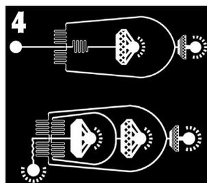
Figure 2, left: Acrylic microfluidic device aimed at exposing and separating the COCs. Figure 3, middle: SEM image of the SU-8 reversible vacuum design. Figure 4, right: Mask designs for microfluidic hydrogel particle maker.
