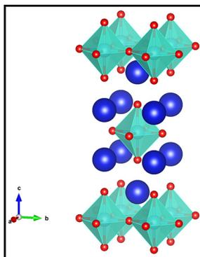
Figure 1: Tetragonal crystal structure of  $\text{Ba}_2\text{RuO}_4$
