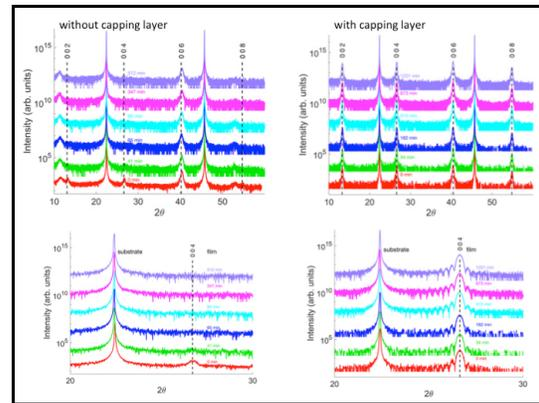
Figure 3: Degradation of  $\text{Ba}_2\text{RuO}_4$  peaks without and with capping layer.
