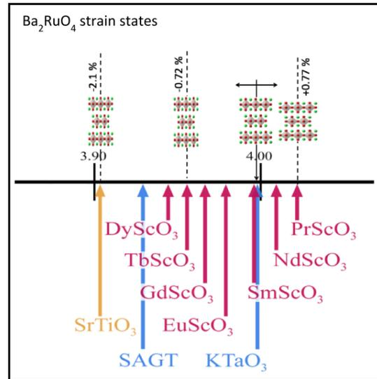
Figure 2:  $\text{Ba}_2\text{RuO}_4$  strain states for various substrates.
