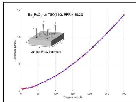
Figure 4: Best  $RRR$   $\text{Ba}_2\text{RuO}_4$  sample from the helium dipper.
