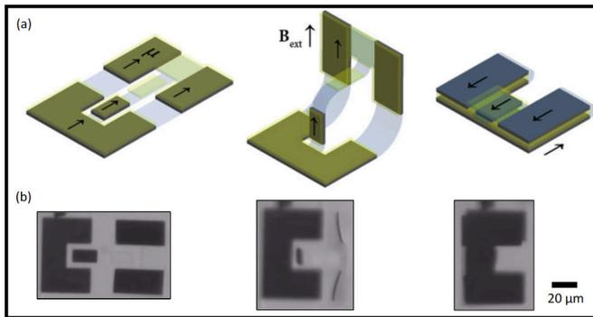
Figure 1: (a) Schematic and (b) optical image of 2D-to-3D magnetically actuated device with latching mechanism —  $\mu$  represents the magnetic moment and  $B_{ext}$  the external magnetic field.
