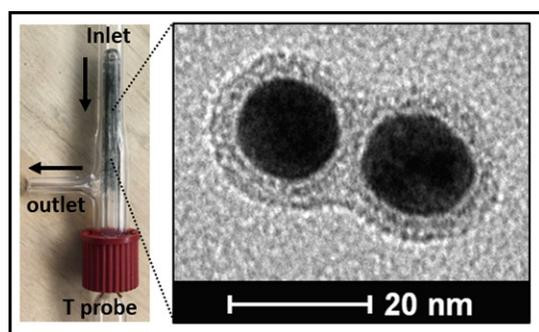
Figure 3: Lab-scale reactor coated with Au-Mo NPs.
