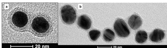
Figure 1: Au NPs with  $(\text{MoS}_2)_2^-$  shell from 6-step (a) and 3-step (b) purification method.
