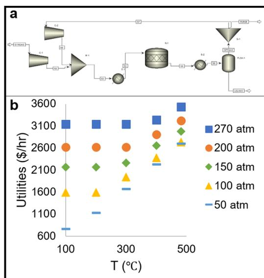
Figure 4: ASPEN model of  $\text{NH}_3$  production (a) and utilities cost at various operating conditions (b).
