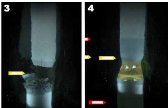
Figure 3, left: Result of the classical floating zone growth attempt at 165 bar. Figure 4, right: Result of the traveling solvent floating zone growth with pure Li<sub>2</sub>MoO<sub>4</sub> at 150 bar.
