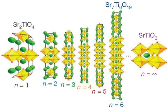
Figure 1 Structure of  $(\text{SrTiO}_3)_n\text{SrO}$ <sup>[1]</sup>
