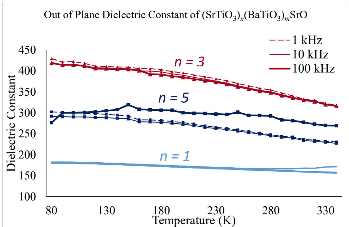
Figure 6: For all of the samples measured, there is no clear peak, and therefore, ferroelectric transition indicated. Compared to in-plane, out-of-plane dielectric constants are much lower.
