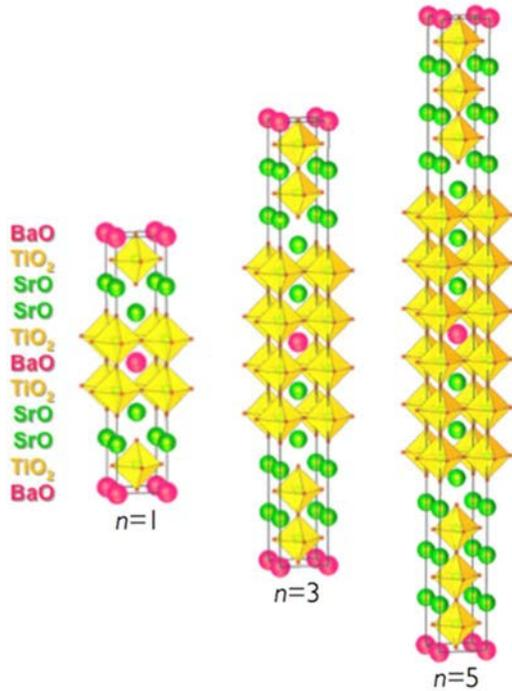
Figure 2 Structure of  $(\text{SrTiO}_3)_n(\text{BaTiO}_3)_m\text{SrO}$ <sup>[2]</sup>
