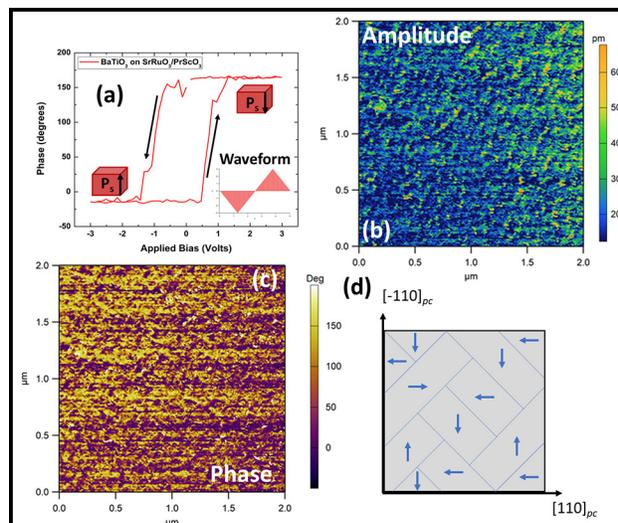
Figure 3, left: Locally poled  $\text{BaTiO}_3$  thin-film, (a) and the written domain wall seen in PFM amplitude, (b). Figure 4, right: Out-of-plane hysteresis (a) of  $\text{BaTiO}_3$  on  $\text{PrScO}_3$ , lateral PFM mapping amplitude response (b), the corresponding phase (c), and a derived model depicting truncated  $aa$ -domains with in-plane polarization (d).
