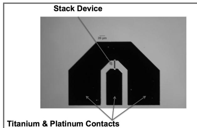
Figure 1: Device geometry used for ST-FMR measurements.
