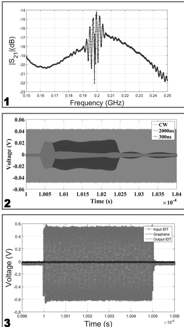
**Figure 1, top:** Plot of frequency domain measurements for gyro device. **Figure 2, middle:** Plot of pulsed wave input time domain measurements for gyro device. **Figure 3, bottom:** Plot of pulsed wave input time domain measurements for graphene device.
