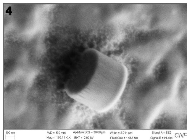
Figure 3, left: SEM of highly uniform  $\text{TiO}_2$  trapezoidal disk nanoparticles fabricated for high force trapping on a waveguide.
