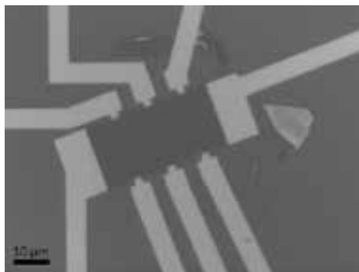
Figure 2: Few layer MoS<sub>2</sub> device fabricated by the authors.
