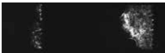
Figure 3: Microscope image of fluorescence on beads after flowing of FITC through chip.
