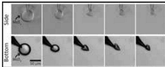
Figure 2: (top) Time lapse of Fluorinert droplet wrapping by MoS<sub>2</sub>, side view; (bottom) Time lapse of the same droplet wrapping, bottom view.
