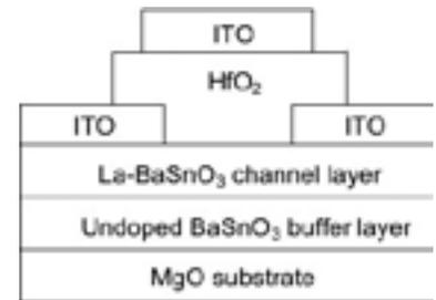
Figure 1: Schematic of the filed effect transistor based on La-BaSnO<sub>3</sub>.
