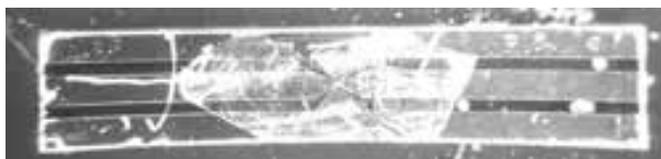
Figure 3: Multilayer graphene deposited on top of a coplanar waveguide spin-coated with a 200 nm thick polystyrene film. See full color version on pages xxviii-xxix.
