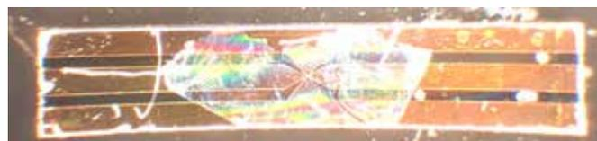
Attoneuton Sensitivity Magnet-Tipped Cantilevers and Sample Preparation for Single-Electron Spin Detection, CNF Project Number: 863-00; Figure 3: Multilayer graphene deposited on top of a coplanar waveguide spin-coated with a 200 nm thick polystyrene film; pages 66-67.
