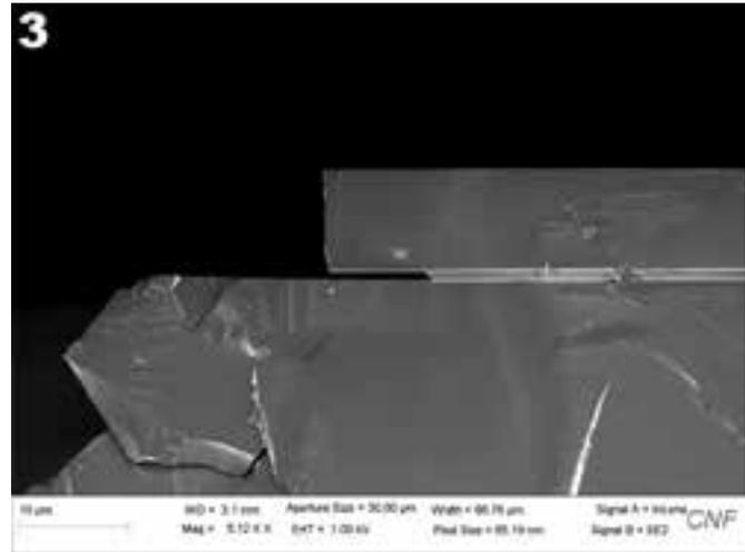
Figure 3, below right: An SEM picture of the partial release of the buried oxide layer of an SOI test sample using the Primaxx vapor HF etch system.
