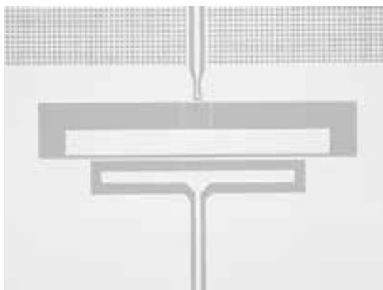
Figure 4: Optical micrograph of superconducting qubit for experiments probing the effects of magnetic flux noise on qubit decoherence.
