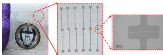
**Figure 2.** Optical images of integrated, transparent, stretchable transistor arrays.
