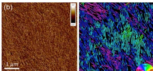
**Figure 1.** AFM phase image of thin film from microfluidic-cooling-UV processed solution. Fibers were extracted and their orientations labeled using GTFiber [[gtfiber.github.io](https://github.com/gtfiber)]
