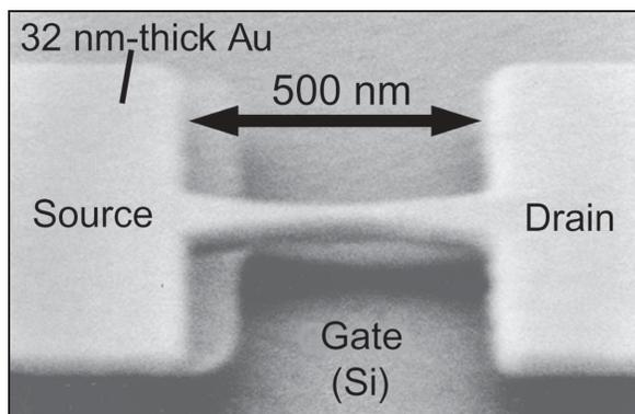
Figure 1: SEM image of a gated-mechanical-break junction before breaking.
