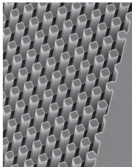
*Figure 2. An SEM image of the DNA purification pillars is shown. Pillars are 10  $\mu\text{m}$  square by 50  $\mu\text{m}$  tall and are coated with  $\text{SiO}_2$  for DNA binding. The array of pillars creates a large surface area for maximum binding of DNA.*
