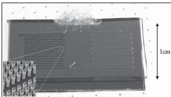
*Figure 1. An integrated microchip for DNA purification and real-time PCR. The inset SEM image shows 10  $\mu\text{m}$  square pillars etched 50  $\mu\text{m}$  into silicon. The pillars are coated with  $\text{SiO}_2$  for DNA binding.*
