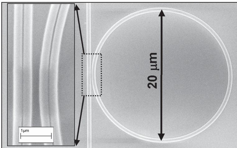
Figure 1: Top-view SEM picture of a ring resonator made of slot-waveguide.
