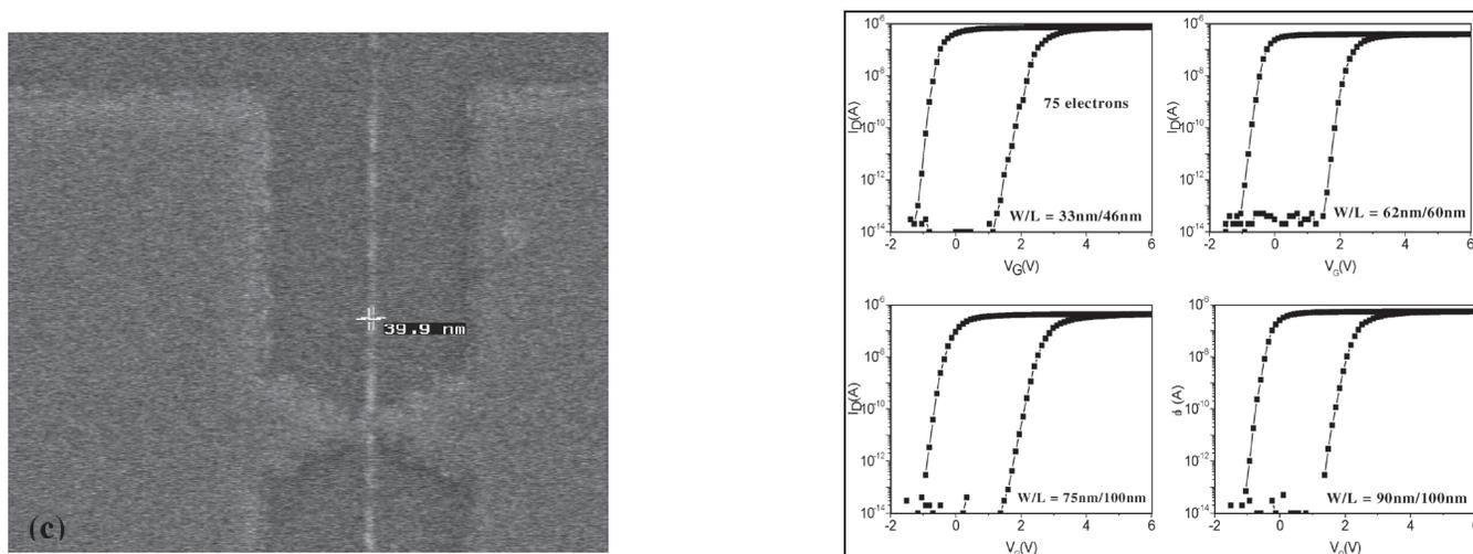
Figure 1: SEM images of a device with width and length of 33 nm and 46 nm.
