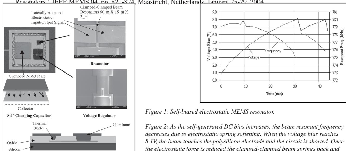
Figure 1: Self-biased electrostatic MEMS resonator.
