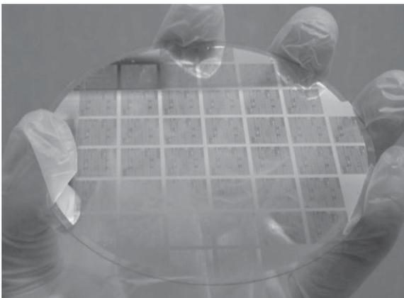
Figure 1: A device layer transplanted onto a glass wafer.
