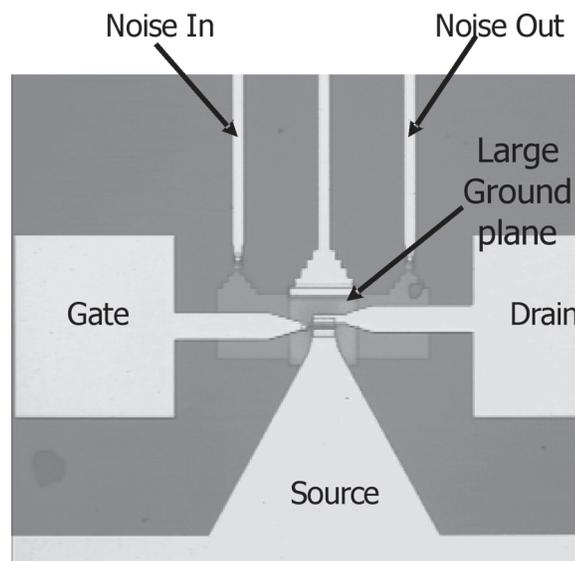
Figure 2: Top-view of a transistor with underlying 3D structure.
