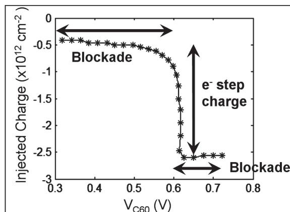
Figure Caption: "Electron injection into C<sub>60</sub> molecules vs potential on C<sub>60</sub> relative to the Si conduction band in a MOS capacitor structure extracted from CV measurements at T=10K showing step-charging."
