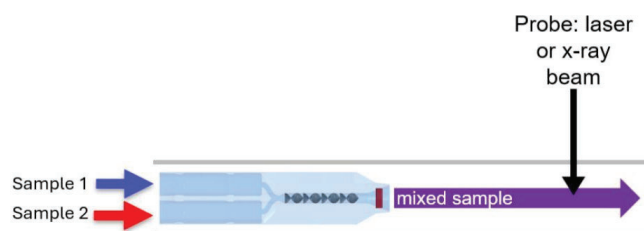
Figure 1: Schematic of a flow cell with a Kenics mixer.
