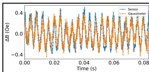
Figure 4: Comparison of measurements of a 251 Hz modulation field with a rms 0.153 Oe from the 4-constriction SHNO sensor and the Gaussmeter.
