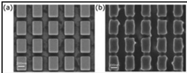
Figure 1: (a) A scanning electron microscope image of a typical a-Si-based resonant metasurface on an ITO-coated  $\text{SiO}_2$  substrate. (b) Same as (a), but before improving the fabrication process.
