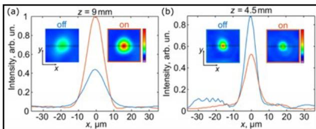
Figure 4: Experimental voltage-dependent focal spot profiles of the metalens (a) Intensity linecuts of the  $z = 9$  mm focal spot image at the 'off' and 'on' voltages of  $2.2V_{pp}$  and  $9.8V_{pp}$ , respectively. The insets show the respective camera images. (b) Same as (a), but for  $z = 4.5$  mm.
