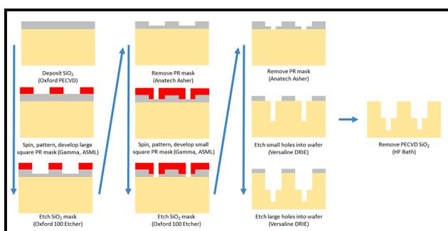
Figure 1: Process flow for fabricating a double-layer ARC on Si wafer.
