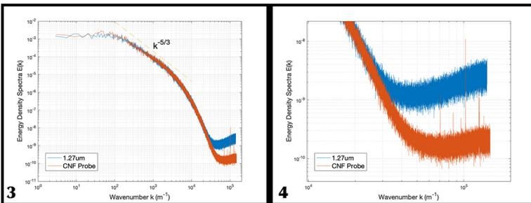
Figure 3, left: Comparison of turbulent spectra from a jet measured with a CNF probe and conventional  $1.27 \mu\text{m}$  hot-wire. We observe a high degree of agreement in the collected spectra. Figure 4, right: Magnified image of the high-frequency spectra. Compared to the conventional hot-wire, the CNF probe is able to resolve more of the dissipation range. The spectra appear to flatten at higher frequencies, most likely due to the noise floor of external electronics.
