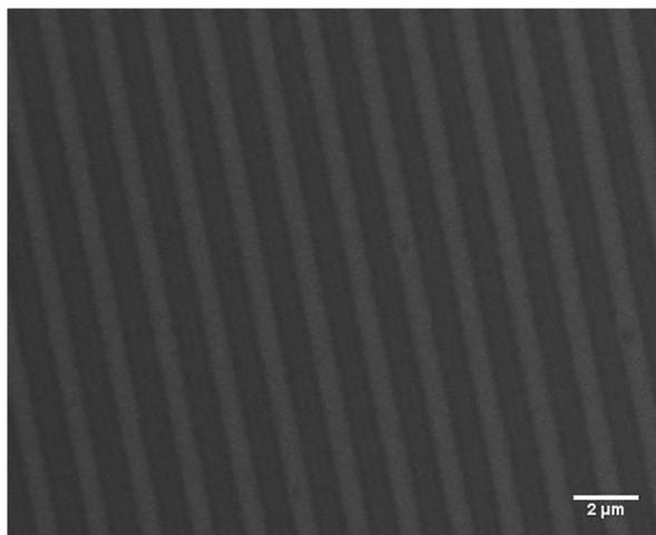
Figure 2. 1:1 Line space pattern with feature size 512 nm observed under SEM after exposure of 100mJ/cm<sup>2</sup> deep UV exposure.
