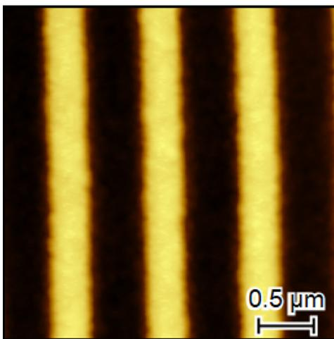
Figure 1. 1:1 Line space pattern with feature size 512 nm observed under AFM after exposure of 100mJ/cm<sup>2</sup> deep UV exposure.
