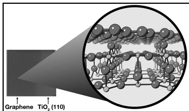
Figure 1: Optical image of TiO<sub>2</sub>(110) with single-layer graphene on left side. The inset is a model of single-layer graphene on TiO<sub>2</sub>(110).
