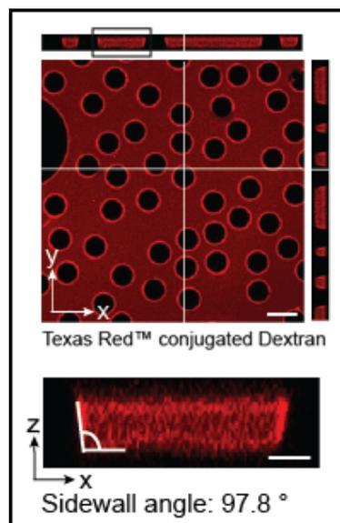
Figure 4: Confocal 3D reconstruction of confined migration area. The PDMS microfluidic device was bonded to a glass coverslip, filled with fluorescent TexasRed-conjugated Dextran, and imaged by confocal microscopy to create a 3D image stacks. Orthogonal projection used to measure sidewall angle,  $\alpha$ , of  $97.8^\circ$ . Scale bars:  $4\ \mu\text{m}$ . Figure adapted from manuscript submitted to *Methods in Molecular Biology*.
