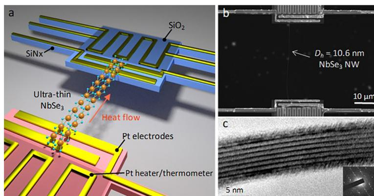
Figure 1: (a) Schematic illustration of the measurement scheme. (b) An SEM micrograph showing a nanowire on the device with a suspended length of  $28.2 \mu\text{m}$ . (c) An HRTEM image of an ultra-thin  $\text{NbSe}_3$  nanowire showing the crystalline structure.
