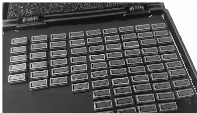
*Figure 4: Example of spectrometer batch made with contract manufacturing process that includes fabrication steps at CNF.*
