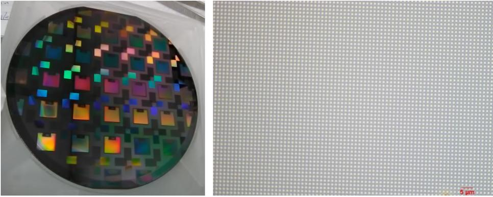
Figure 2, left: Wafer lithographically patterned with optical metastructures, using the ASML DUV stepper, Figure 3, right: Optical microscope image of test pattern of array of  $\sim 1 \mu\text{m}$  pillars, also patterned on the ASML.
