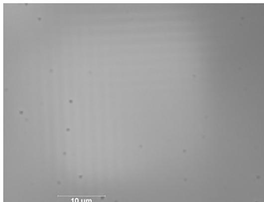
Figure 2: Optical microscope images of patterned film with 150. Prebake: 150°C/60s; Exposure: 20 mJ/cm<sup>2</sup>; Development: isopropanol 120s.
