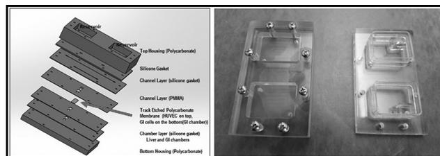
Figure 1: Design of the two-chamber unidirectional device for liver metastasis. Schematic view and actual photographs of the assembled frames.
