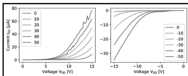
*Figure 1: I-V curve for FET made from lead halide perovskite (FAMACs) on substrates fabricated at the CNF. Source-to-drain current ( $I_{SD}$ ) versus source-to-drain voltage ( $V_{SD}$ ) at different source-to-gate voltages ( $V_G$ ). Gate voltage sweep direction: 0 V to 50 V and 0 to -50 V.*
