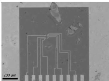
Figure 1: Spin-coated 380 nm ionic gel on MoS<sub>2</sub> few-layer device. Large surrounding metallic region is Pt gate, bars at bottom of image are optically patterned leads to bond pads.
