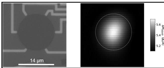
Figure 2: Left, optical image of few layer MoS<sub>2</sub> device fabricated by the authors. Right, magnetic susceptibility map of the same device, as acquired by scanning SQUID microscope.
