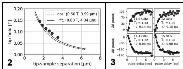
**Figure 2, left:** Tip field versus tip-sample separation along with a fit to an analytical magnet field for a spherical model. **Figure 3, right:** Cantilever phase shift versus pulse delay measured at different irradiation frequencies. Inset shows best fit spin-lattice relaxation time.
