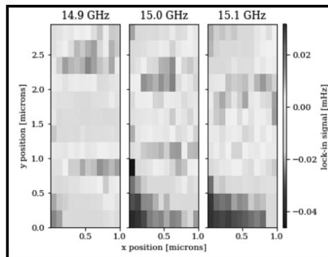
**Figure 4:** Map of spin-induced cantilever frequency shift at various irradiation frequencies. Step size:  $\Delta x = 91$  nm,  $\Delta y = 258$  nm. (See pages vi-vii for full color version of figure.)
