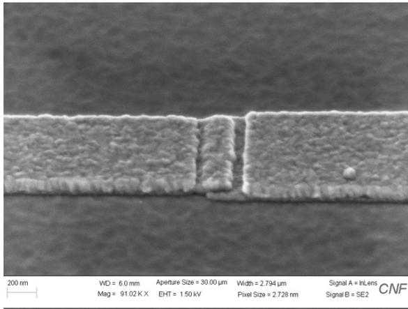
Figure 1: Scanning electron micrograph of Al-AlO<sub>x</sub>-Al Josephson junction for superconducting qubit.
