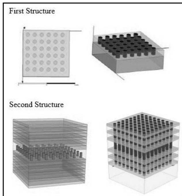
Figure 1: First Structure: The 1.5  $\mu\text{m}$   $\text{SiO}_2$  film was deposited, patterned and etched. The holes were 0.5  $\mu\text{m}$ , electroplated with Cu. Second Structure: Alternative layers of  $\text{SiO}_2$  and Si are deposited, patterned and etched (all through the layers), then holes electroplated with Cu.
