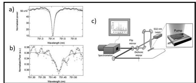
Figure 1: a) Ring resonance at 751.41nm with  $Q = 350,000-200,000$ . b) Ring resonance after monolayer transfer with  $Q = 95,000$ . c) Experimental setup to pump from the top and collect the chip's output from the side.
