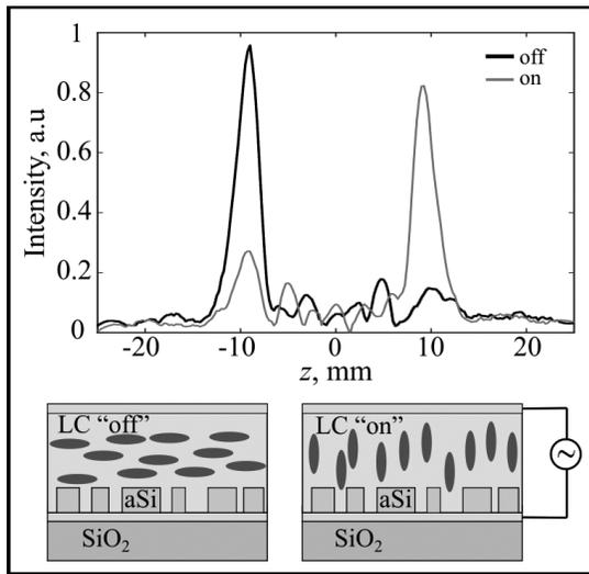
Figure 2: Top, simulated intensity of light transmitted through the  $\alpha$ -Si metalens, plotted along the optical axis of the lens. The lens acts as a converging lens with +8 mm focus in the absence of an external electric field (black line) and acts as a diverging lens with a -8 mm focus in the presence of an external electric field (light gray line). Bottom, schematic of an  $\alpha$ -Si metalens design.
