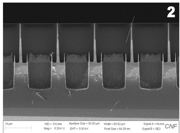
**Figure 1, top:** Process flow for fabricating a double-layer ARC on a silicon wafer. **Figure 2, bottom:** SEM image taken using CNF's Zeiss Ultra SEM showing the two-layer structure of anti-reflection coatings.
