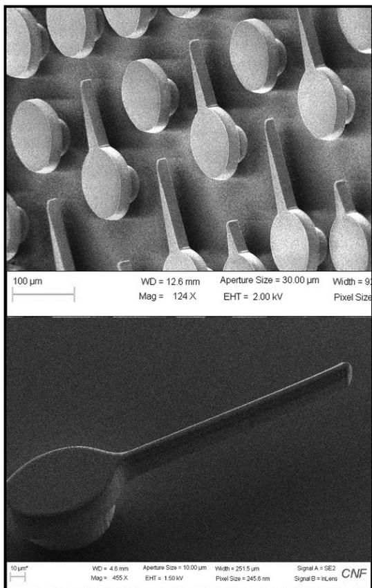
Figure 2: SEMs of SU-8 microcantilevers on glass slides.
