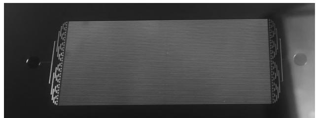
Figure 3: Etched silicon mold for hot pressing.
