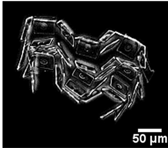
Figure 3: A spacer Miura-ori fold made using ultra-thin, self-folding atomic layer deposited sheets.
