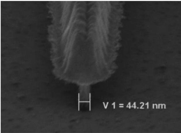
Figure 1: T-gate demonstrating a gate length of 44 nm.
