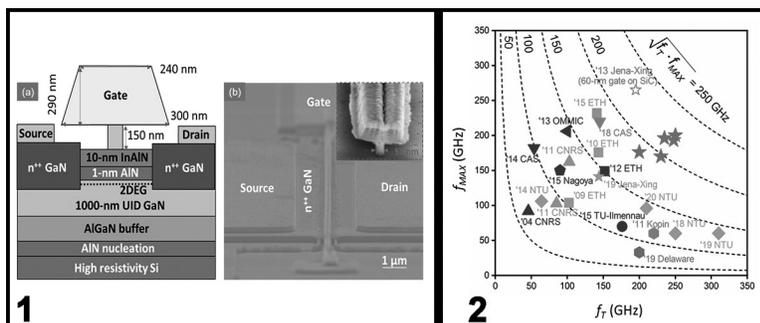
**Figure 1, left;** (a) Schematic cross-section of InAlN/AlN/GaN HEMTs on Si with regrown  $n^+$ GaN contacts. (b) An angled SEM image of a fabricated InAlN/AlN/GaN HEMT with an EBL T-gate. **Figure 2, right;** Comparison of the measured  $f_T$  and  $f_{MAX}$  of GaN HEMTs on Si substrates. (See pages vi-vii for full color versions.)
