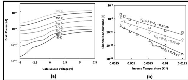
Figure 3: (a) Transfer characteristics of a PtSe<sub>2</sub> MOSFET at different temperatures. (b) Channel conductance of a PtSe<sub>2</sub> MOSFET between 80 and 290 K.
