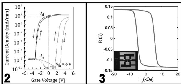
Figure 2, left:  $I_d$ - $V_{gs}$  and  $I_d$ - $V_d$  characteristics of the  $\text{LuFeO}_3$ -GaN Fe-FET device, showing 2DEG depletion and hysteretic behavior, as well as saturation. Figure 3, right: Hall resistance of Pt/ $\text{Mn}_4\text{N}$  Hall bar (Inset: photo of the measured device).
