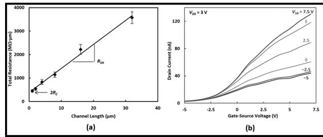
Figure 2: (a) TLM results. (b) Transfer characteristics of a PtSe<sub>2</sub> MOSFET under different source contact biases.
