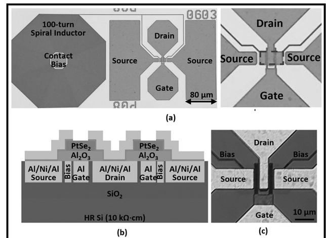
Figure 1: (a) Optical micrograph of individually probable RF MOSFET with source contact biased through a spiral inductor. (b) Cross section schematic. (c) Top-view micrograph of a finished PtSe<sub>2</sub> MOSFET.
