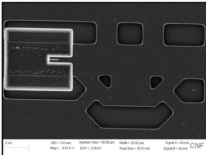
Figure 1: Magnet-on-chip design with an e-beam patterned cobalt. This specific pattern has a magnet of  $\sim 1 \mu\text{m}$  in length,  $80 \text{ nm}$  in width and  $200 \text{ nm}$  in thickness. The overhang is  $\sim 230 \text{ nm}$ .
