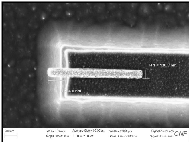
Figure 2: Cobalt magnet overhanging at the edge of the chip design. The magnet patterned is  $\sim 1.2 \mu\text{m}$  long,  $136 \text{ nm}$  wide and  $200 \text{ nm}$  thick. The overhang is  $294 \text{ nm}$ .
