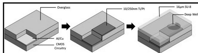
*Figure 1: The geometry of shift electrode. The opening of the working area is redefined. In our case, one passivation SU-8 layer is applied with redefined shape (round) of the new opening for better cell trapping.*
