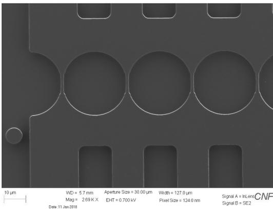
Figure 2: SEM image of a row of  $1\mu\text{m}$  constrictions created by etching  $5\mu\text{m}$  into silicon by deep-reactive ion etching.
