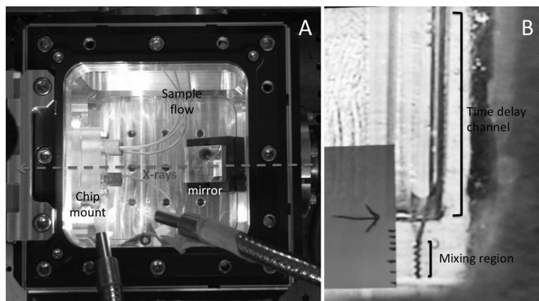
Figure 1: Microfluidic mixing chip for SAXS mounted *in vacuo* at CHESS beamline G1. A: X-rays (red) pass through cubic vacuum enclosure over viewing mirror and through microfluidic cell. B: Mixing region and time-delay channel of chip are visible in camera snapshot.
