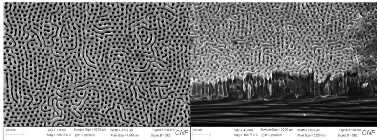
Figure 4: SEM micrograph of BCP on 50 nm of SiO<sub>2</sub> on Si after CH<sub>2</sub>F<sub>2</sub>/He and HBr/Ar etch. Left: Top down. Right: Cleaved, 45 degrees.
