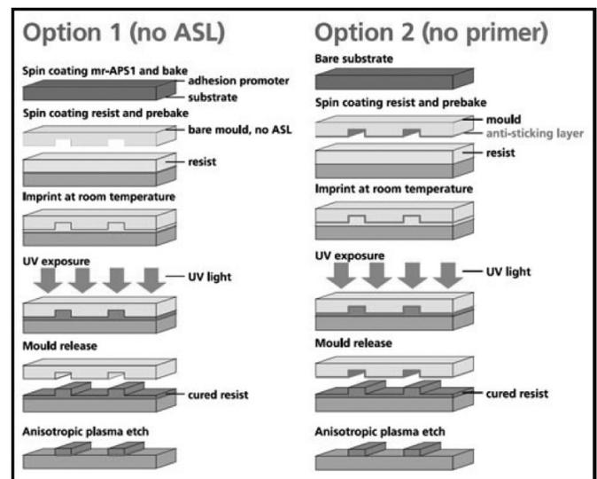
Figure 1: mr-XNIL26 P-NIL process overview from Microresist Technology.
