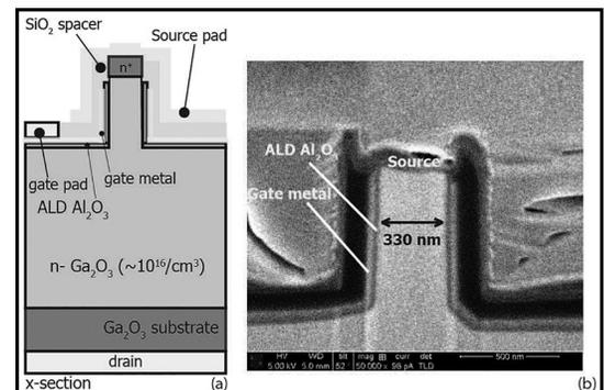
Figure 1: (a) Schematic cross-section of a Ga<sub>2</sub>O<sub>3</sub> vertical power MISFET. (b) 52° SEM cross-section image of a completed Ga<sub>2</sub>O<sub>3</sub> vertical Fin-MISFET showing a 330 nm wide and 795 nm long channel.
