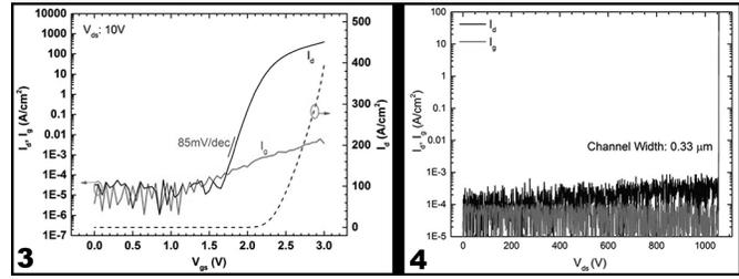
Figure 3, left: Representative *I<sub>d</sub>*/*I<sub>G</sub>*-*V<sub>gs</sub>* transfer characteristics in the semi-log and linear scale, along with the extracted subthreshold slope. Figure 4, right: Representative three-terminal off-state (at *V<sub>gs</sub>* = 0 V) *I<sub>d</sub>*/*I<sub>G</sub>*-*V<sub>ds</sub>* characteristics and breakdown voltage of Ga<sub>2</sub>O<sub>3</sub> vertical power MISFETs.
