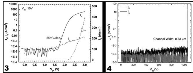
**Figure 3, left:** Representative *I<sub>d</sub>*/*I<sub>s</sub>*-*V<sub>gs</sub>* transfer characteristics in the semi-log and linear scale, along with the extracted subthreshold slope. **Figure 4, right:** Representative three-terminal off-state (at *V<sub>gs</sub>* = 0 V) *I<sub>d</sub>*/*I<sub>s</sub>*-*V<sub>ds</sub>* characteristics and breakdown voltage of Ga<sub>2</sub>O<sub>3</sub> vertical power MISFETs.
