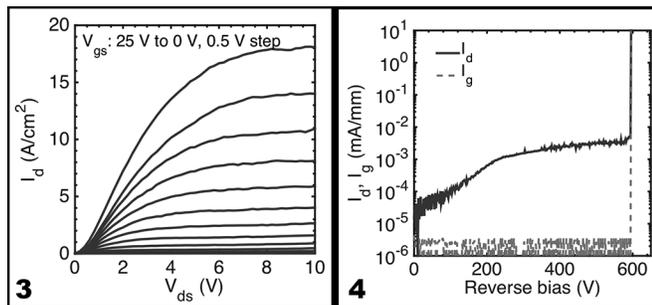
Figure 3, left: Representative  $I_d$ - $V_{ds}$  characteristics of a Ga<sub>2</sub>O<sub>3</sub> vertical power MISFET. Figure 4, right: Representative three-terminal off-state (at  $V_{gs} = -15$  V)  $I_d/I_g$ - $V_{ds}$  characteristics and breakdown voltage of Ga<sub>2</sub>O<sub>3</sub> vertical power MISFETs.
