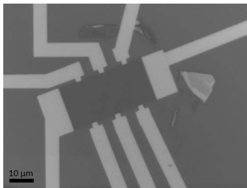
Figure 2: Few layer  $\text{MoS}_2$  device fabricated by the authors.
