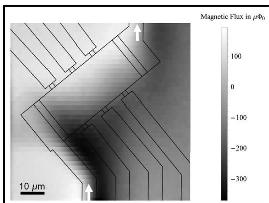
Figure 3: Scanning SQUID image of ionic liquid gated, metallic MoS<sub>2</sub> device. White arrows indicate current source and drain, black outline is device shape. Sample temperature approximately 10 Kelvin.
