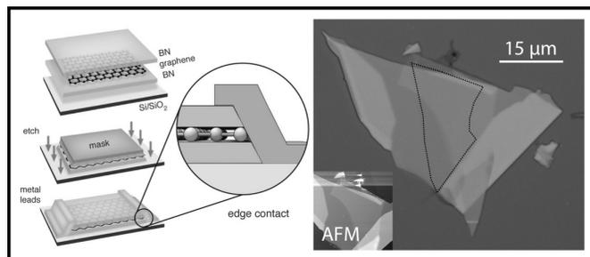
Figure 1: Left panel: overview of process from [3], used with permission. Right panel: a monolayer graphene flake (dotted outline) sandwiched between flakes of hexagonal boron nitride. Inset: AFM image, scaled down.
