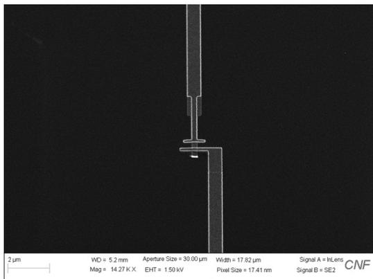
Figure 3: Scanning electron micrograph of cross-style Al-AIO<sub>x</sub>-Al Josephson junction for superconducting qubit patterned on the JEOL 9500.
